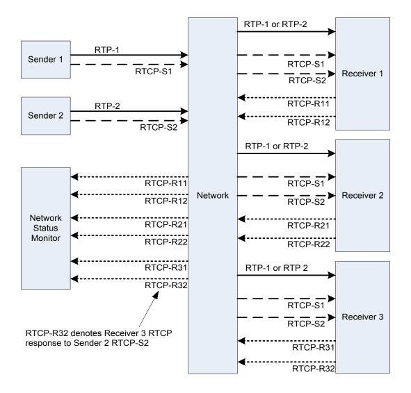
Figure 2: Example System for RTCP Receiver Selection Signaling
