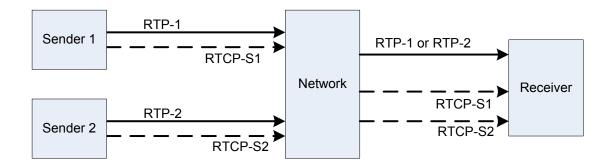
Figure 1: Example System for RTCP Redundancy Signaling
