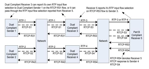
Figure 6: Example System for Dual Compliant Devices
